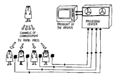
Cable television companies are now experimenting with several kinds of interactive systems. Subscriber Response Systems (SRS) enable a single computer to collect information from the terminals of ten thousand subscribers in less than two seconds.
